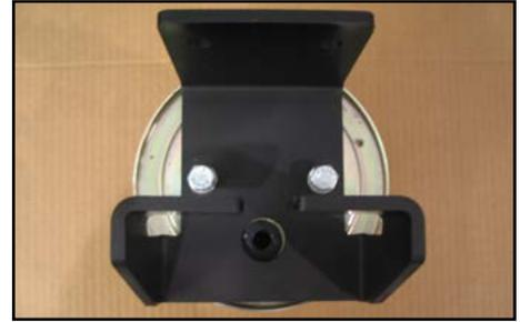
Install and tighten the 90° airline fitting in to the air spring using thread sealant.
