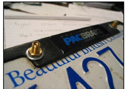
NOTE: This kit contains push to connect fittings, using scissors or wire cutters to cut the nylon airline will distort the line and cause the connection to leak. THE AIRLINE MUST BE CUT OFF SQUARELY WITH A SHARP RAZOR KNIFE. Moisten the end of the airline prior to inserting it into the fitting and push it in until it stops.
