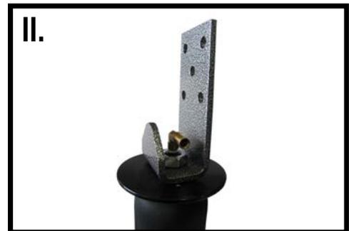
III. Loosely attached the lower bracket to the bottom of the air spring using a 1/2" flat washer and 1/2" -13 x 7/8" hex head cap screw.
