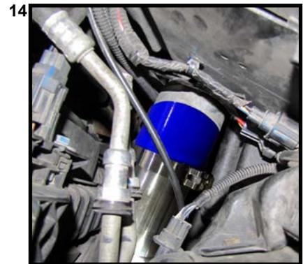
**15** Attach a 3" clamp onto the exposed end of the CAC pipe.
