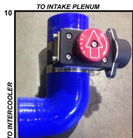
**12** Attach the provided 3" silicone hose to the end of the CAC pipe. Install a provided 3" clamp and torque to 75 in-lbs (8.5 N•m).
