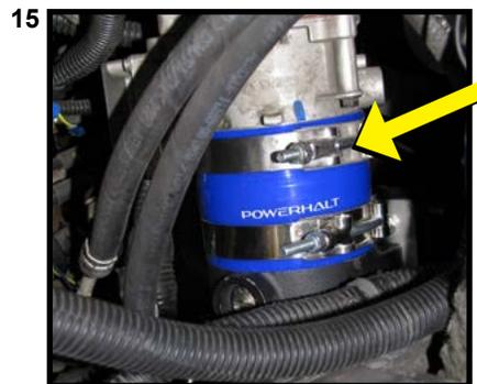
**16** Connect the metri pack connector of the harness to the mating connector on the PowerHalt.
